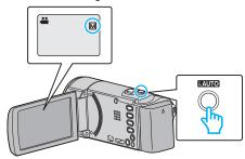
If the mode is i.A. Intelligent Auto, press the i.AUTO button to switch to M Manual.
